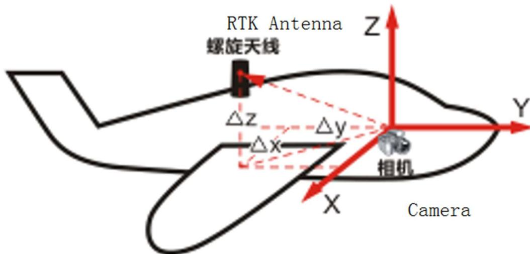
The offset from RTK antenna phase center and camera CMOS center in the body system can be define as below:
