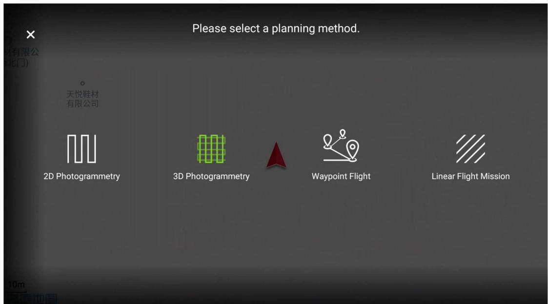
2) Import a KML file or set a mission area manually, double grid airline will be generated automatically.
