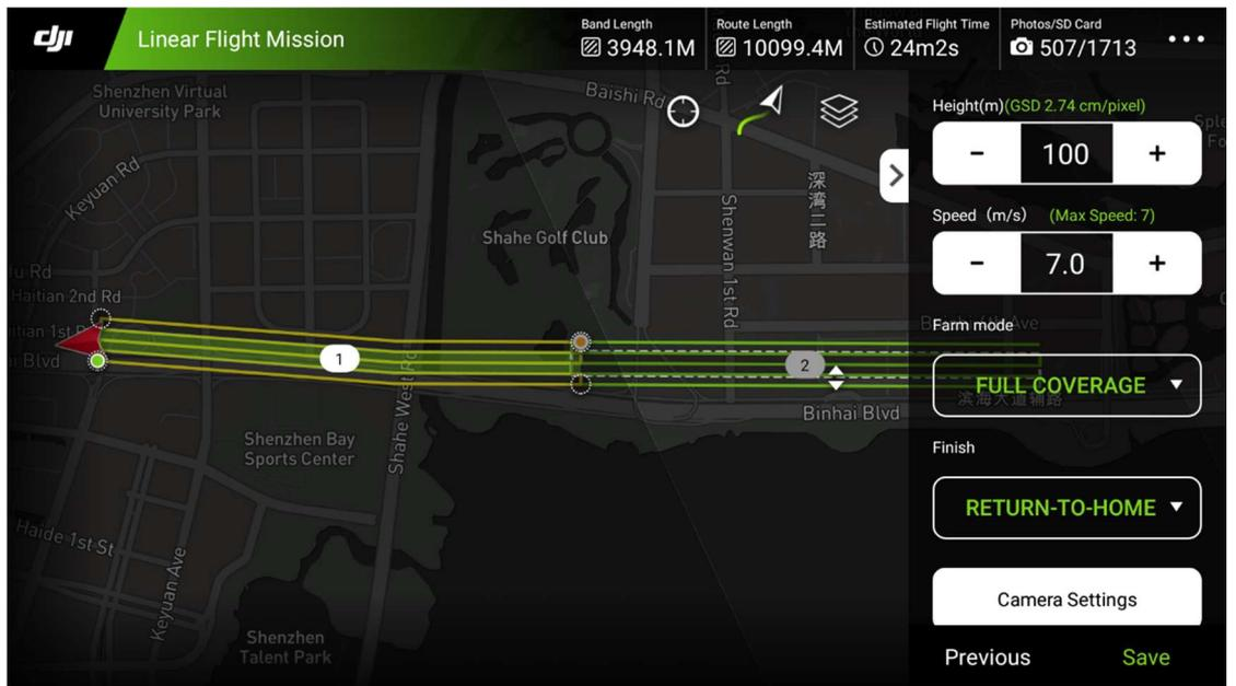
6) There are two modes in the linear flight mode: Full Coverage and Efficiency. “Full coverage” mode has 1 or 2 airlines more than Efficiency mode.
